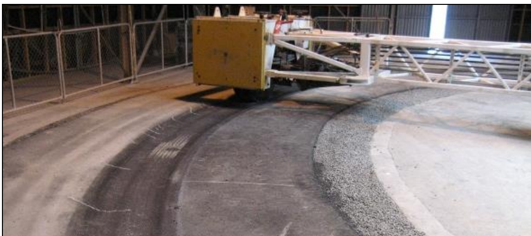
Figure 19: CAPTIF Testing for the Gonzalez FBS Accelerated Loading Experiment
